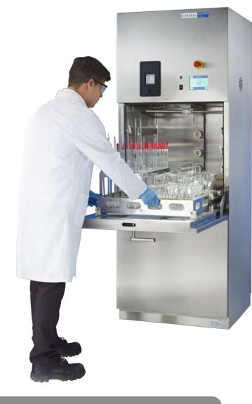
The M-56 spindle rack can process smaller 50 ml glassware.
